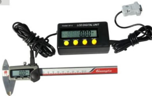
**811-1型液晶显示仪** 811-1 LCD Display Unit
